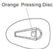
Figure 2: Schematic drawing of PCA button Note: The orange pressing disc must be removed prior to use, otherwise flow rate will be too fast.
